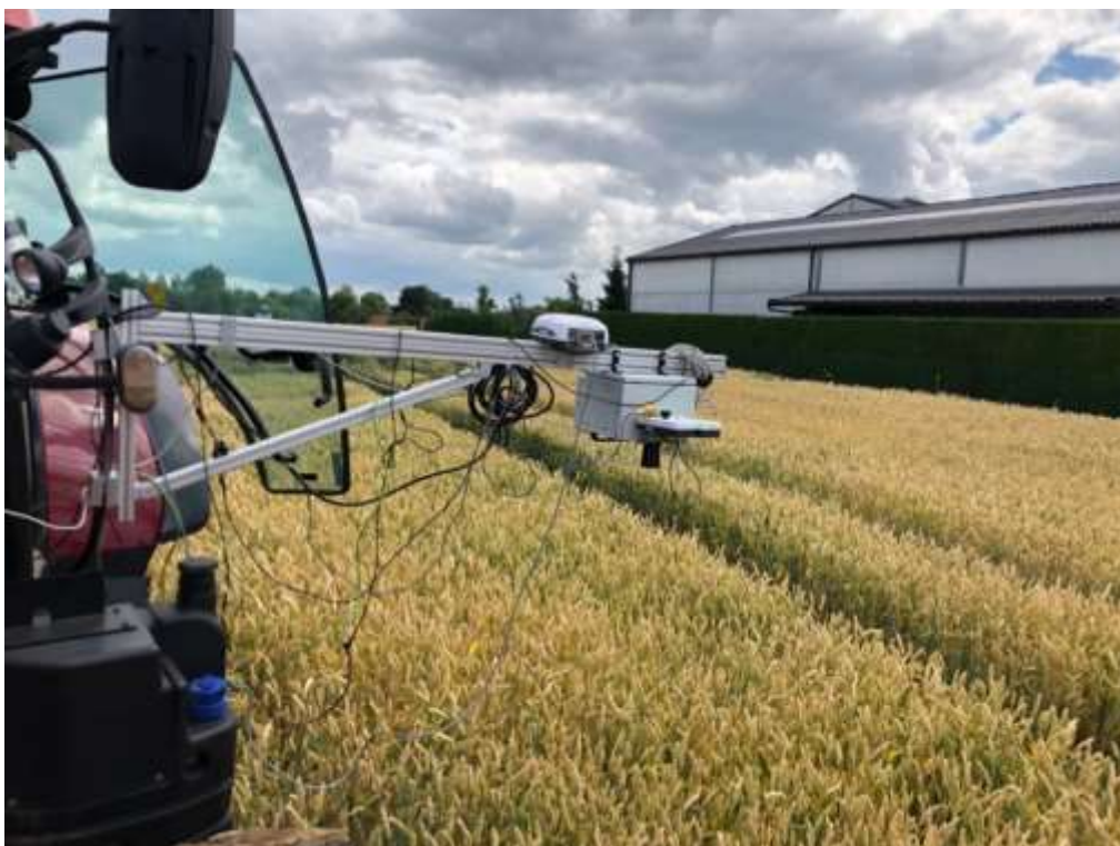
Figure 1. The custom-built metal frame, attached to a tractor during on-line measurements using a multi-sensor box.
