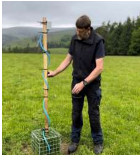
Figure 1: Donald Barrie (Farm manager) demonstrating the use of soil sensors at the case study in Glensaugh, the United Kingdom.
